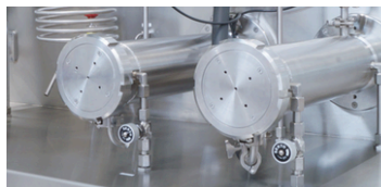
Scraped Surface Heat Exchangers (Cooling to -15°C, -8°C) @ 15L/hr
