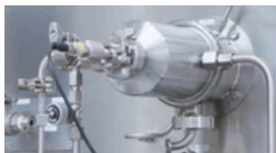
Pin Worker / Kneading (300-2200 RPM)
