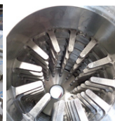
Mixing Head / Air Whipping (300-1500 RPM)
