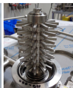
Mixing Head / Air Whipping (300-1500 RPM)
