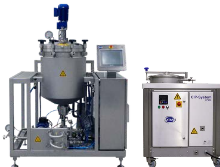
Production line Batch Cooker & CIP250
