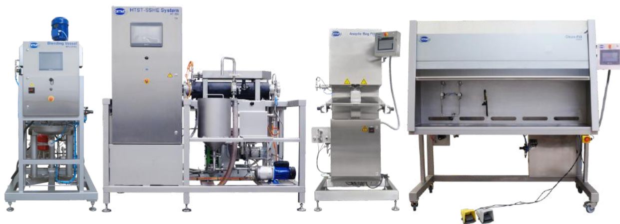
Production line with blending vessel, UHT system, aseptic bag filler & Clean-Fill
