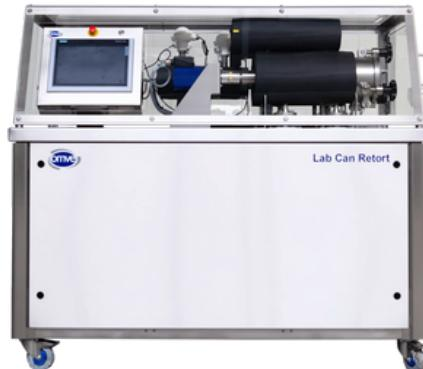
With advanced data logger and intelligent controls, the units make it easy to conduct heat penetration and temperature distribution tests for shelf-stable low-acid canned foods and beverages. This enables the assessment of new packaging materials and food containers to determine optimal processing conditions and recipe validation. With a compact design, food developers can achieve sustainability and innovation efforts.
