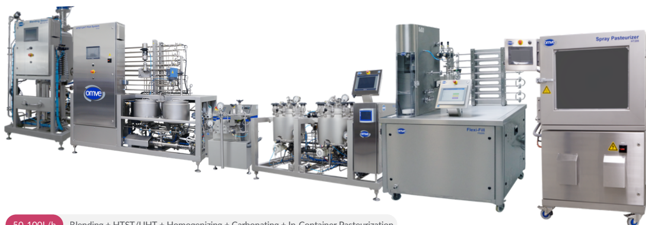
50-100L/h Blending + HTST/UHT + Homogenizing + Carbonating + In-Container Pasteurization
