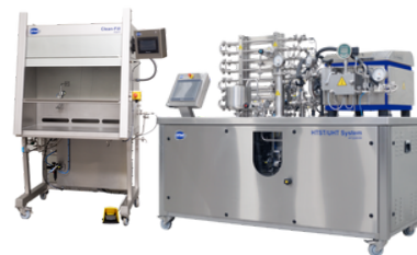
20L/h HTST/UHT Direct & Indirect + Homogenizing + Filling
