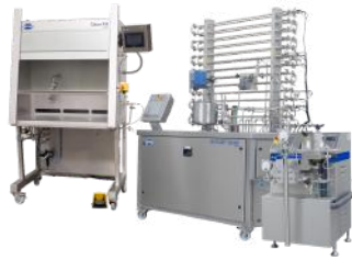
50L/h HTST/UHT + Homogenizing + Filling
