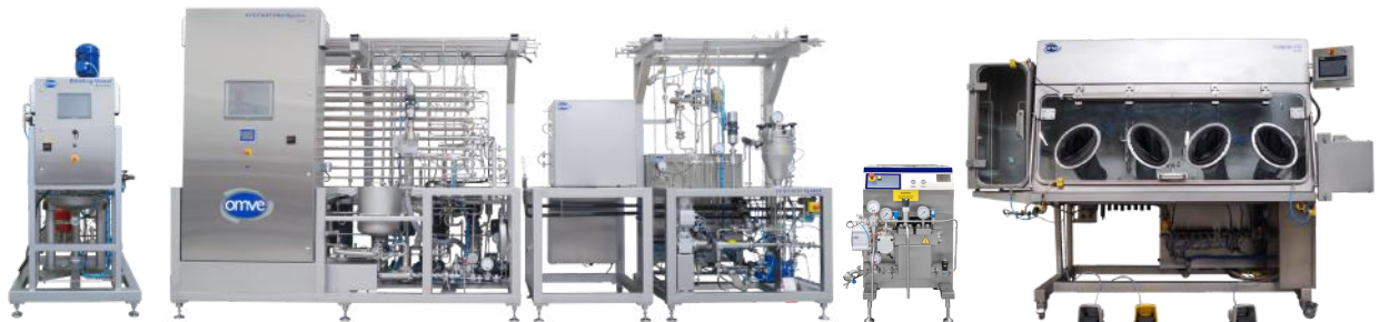
100L/h Blending + Indirect HTST/UHT + Hold tubes + Direct UHT, Homogenizing, Aseptic Filling
