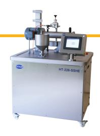
The OMVE SSHE is unique in their hygienic execution. This assures a good cleaning during CIP and minimise contamination during processing. The barrels can also be disassembled for manual cleaning. With the special bearing and high-pressure seals, the SSHE can handle a pressure up to 10 bar. This makes the system especially suitable for very high viscous products and simulates industrial processes where high pressures are preferred.
