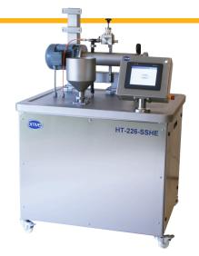
The OMVE SSHE is unique in their hygienic execution. This assures a good cleaning during CIP and minimise contamination during processing. The barrels can also be disassembled for manual cleaning. With the special bearing and high-pressure seals, the SSHE can handle a pressure up to 10 bar. This makes the system especially suitable for very high viscous products and simulates industrial processes where high pressures are preferred.
