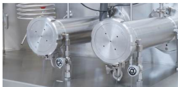
Scraped Surface Heat Exchangers (Cooling to -15^{\circ}\text{C} , -8^{\circ}\text{C} ) @ 15L/hr
