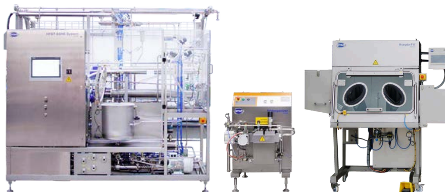
50L/hr HTST/UHT + Homogenizing + Filling
