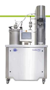
The advanced engineering of the CF210 series allows for precise carbonation control, capable of dissolving up to 11g/I of  $CO_2$  in liquid. This feature provides R&D teams with the versatility to experiment and innovate with new beverage concepts. With user-friendly touchscreen controls, users can effortlessly set and store different carbonation and filling scenarios, streamlining the R&D process.
